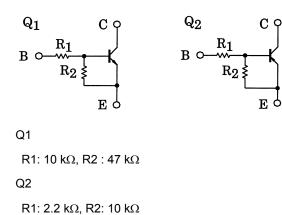
Q1: RN1107F Equivalent Q2: RN2327A Equivalent
